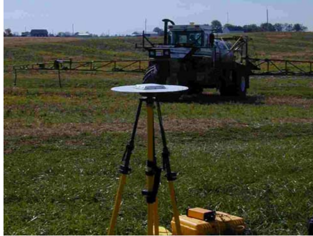
Figure 2. View of RTK base station and Terragator
